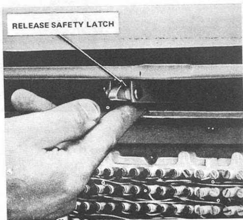
Fig. 3—Releasing Safety Latch
