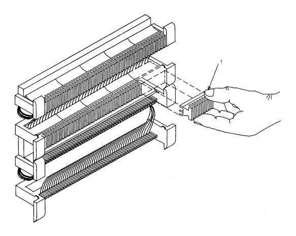
Step 21—Placing 108 Connecting Block Into Index Strip
