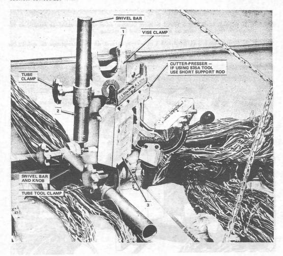
Step 15-Set Up Cutter-Presser on 710A Tool for Splicing
