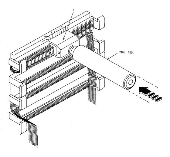
Step 20—Seating and Trimming Conductors
