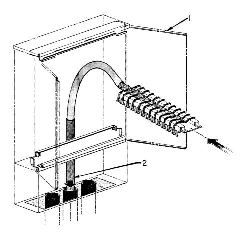
Step 9-Installing Terminal Block in Cabinet
