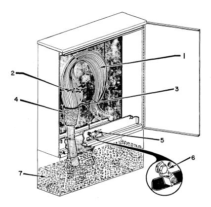
Step 2—Cable Sheath Preparation (Buried Installation)
