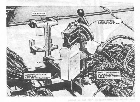
Step 14—Set Up Cutter-Presser on 117A Bracket for Splicing
