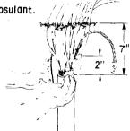
Step 3—Installation of Bond Clamp and Moisture Plug
