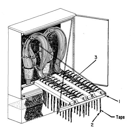
Step 18-Placing Binder Groups Through Wiring Slots
