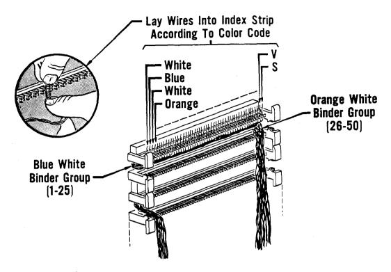
Step 19—Placing Conductors Into Index Strip
