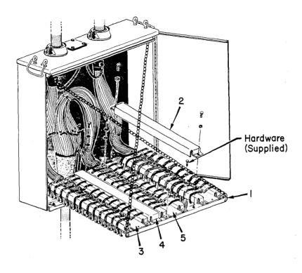
Step 12—Securing Prewired Terminal Block to Frame (Aerial Installation)
