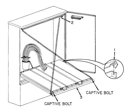
Step 4—Installation of Mounting Frame
