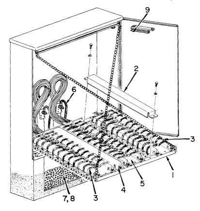
Step 10—Securing Prewired Terminal Block to Frame
