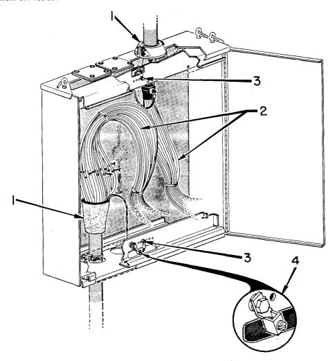
Step 6—Cable Sheath Preparation (Low Pole Mount)
