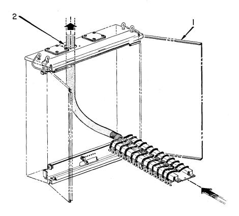
Step 11—Installing Terminal Block in Pole or Wall Mounted Cabinet
