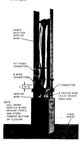
Fig. 28—Service Wire Installed
