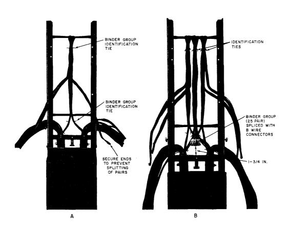
Fig. 23—Completed Binder Group (25 Pairs)
