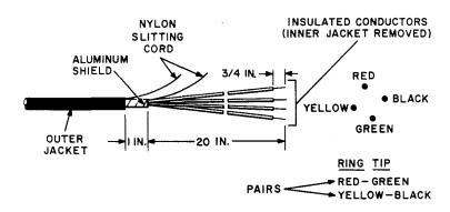
Fig. 26—Preparation of B Service Wire
