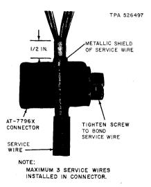
Fig. 27—Installing Service Wire in AT-7796X Connector
