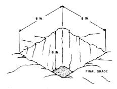
Fig. 14—LD6/42 or LE6/42—Excavation Dimensions
