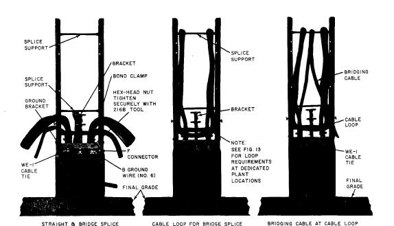
Fig. 21—Cable Installed in Closure
