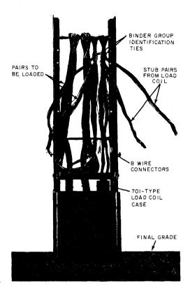
Fig. 29-Load Coil Case Placed
