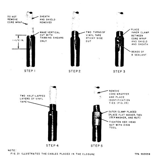
Fig. 20—Installing Bond Clamp—Corrosive Area
