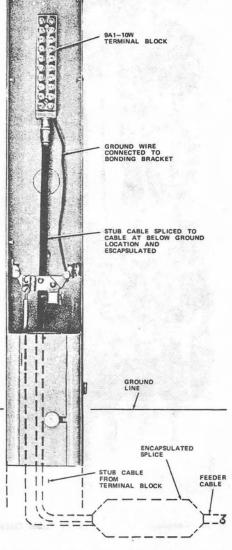
Fig. 25—Closure Used at Junction of Buried and Aerial Plant
