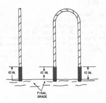
Fig. 16-Cable Sheath Removed
