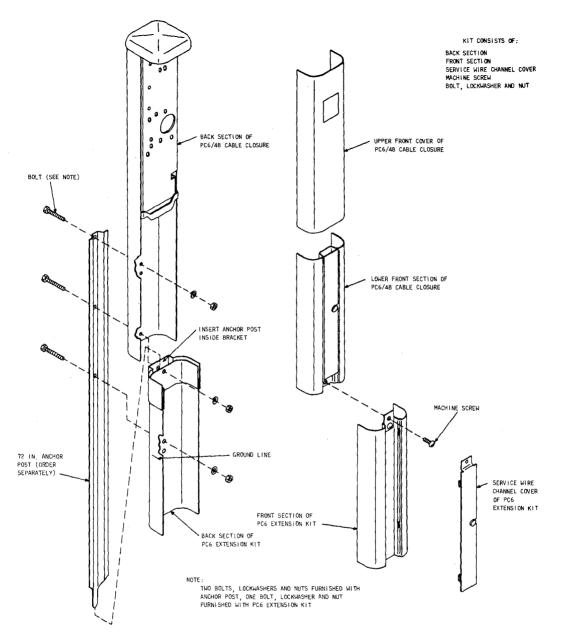
Fig. 15—♦Installation of PC6 Extension Kit♦
