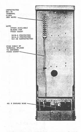
Fig. 21—PC12/55 Cable Closure Equipped With 9A-Type Terminal Block
