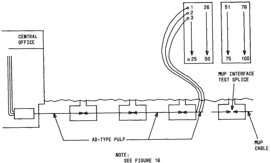
Fig. 15—AD-Type Pulp Cable With MUP Cable
