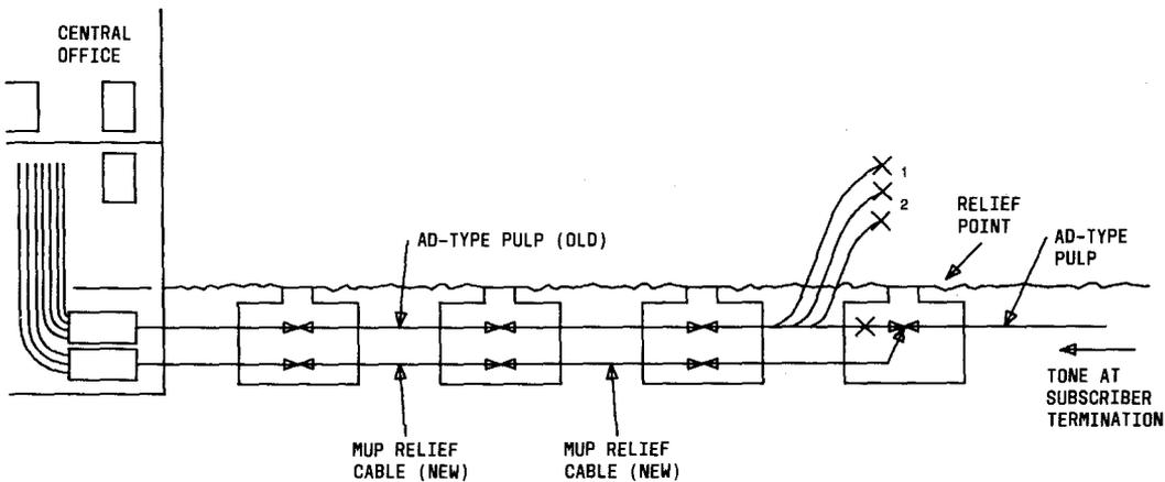
Fig. 14—Working Cable Replaced with MUP Cable
