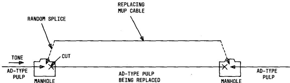
Fig. 13—Replacing AD-Type Pulp Cable With MUP Cable
