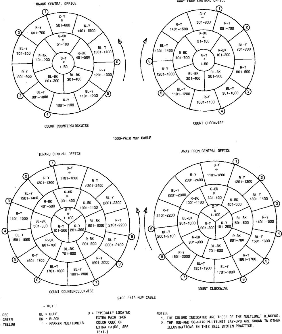
Fig. 9—Cable Count—Typical Straight Splice
