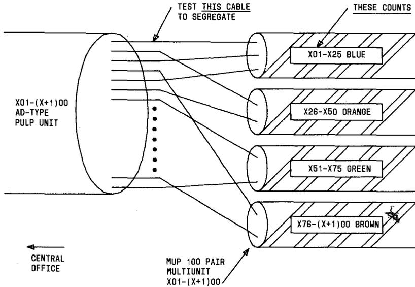
Fig. 16—Testing AD-Type Pulp Interfaces
