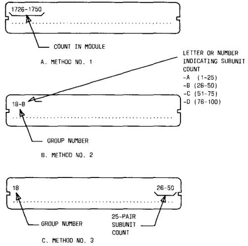
Fig. 11—Various Methods for Marking Module
