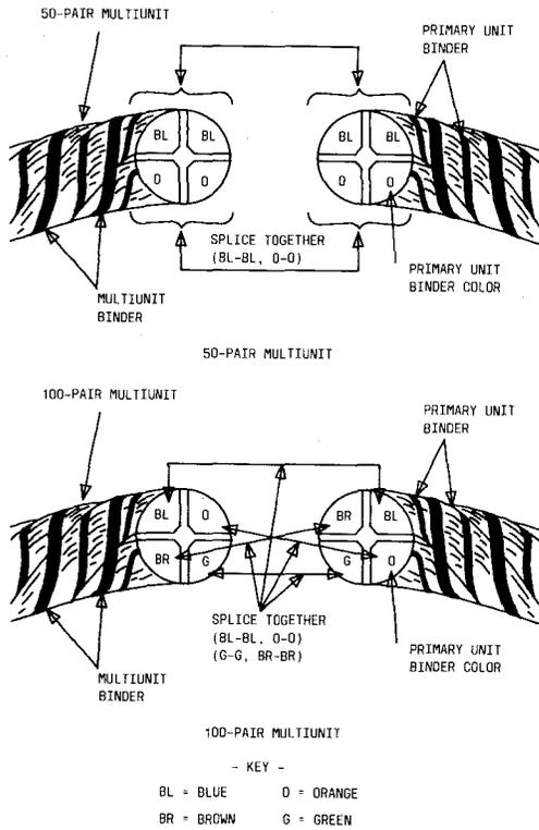
Fig. 10—Color-to-Color Splicing of MUP Primary Units
