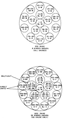
Fig. 8—Superseded 200- and 600-Pair Alternate Core Makeups
