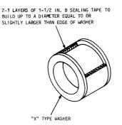
Fig. 9—HX, JX, and KX Sealing Washers for Sealing Vacant Opening in End Plate
