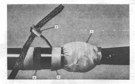
Fig. 19-Completed Wrapped Joint
