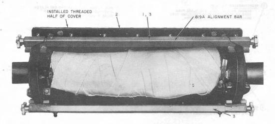
Fig. 44—Installing Cover Halves
