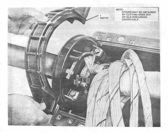
Fig. 36-Securing Cover Half
