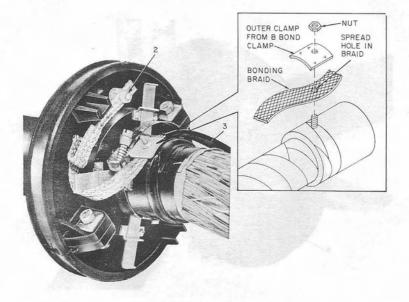
Fig. 24—Attaching Bonding Braid
