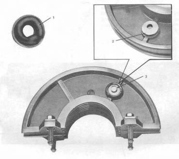
Fig. 41—Installed Repair Washer on End Plate
