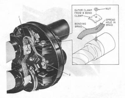
Fig. 28—Attaching Bonding Braid
