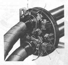
Fig. 27-Installation of B Bond Clamp and Sealing Clamp
