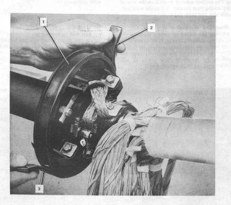
Fig. 34—Placing 3/4 Inch Wide  $\times$  1/4 Inch Thick B Sealing Tape in Groove of End Plate
