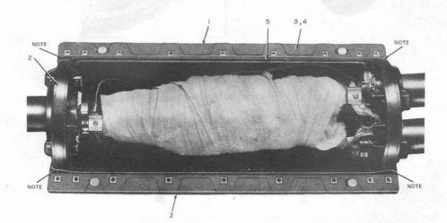
Fig. 42-Placing Cover Halves Using B Sealing Tape and Cord
