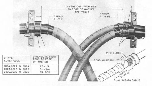
Fig. 20-Installation of B Sealing Tape Collars
