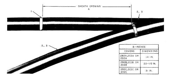
Fig. 14—Mark Cable Sheath and Remove Polythylene Jacket and Flooding Compound
