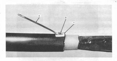
Fig. 17-Bonding Cable Sheath
