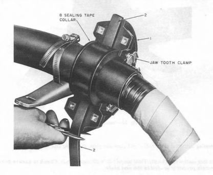
Fig. 21—Placing Threaded Insert Section of End Plate
