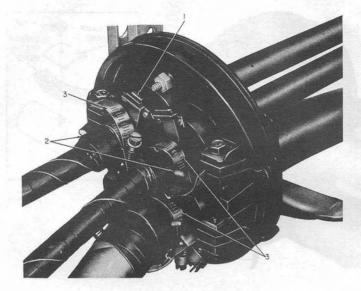
Fig. 31—Installation of B Bond Clamp and Sealing Clamp
