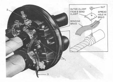
Fig. 32—Installed Bonding Braid
