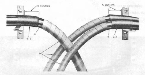
Fig. 12—Prepared Cable Sheath
