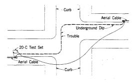
Fig. 3—Direct Connection At Two Points
