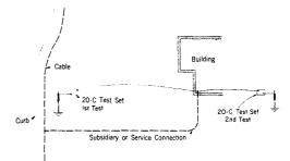
Fig. 6-One Direct Connection and One Ground Rod
