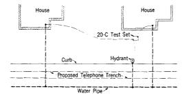
Fig. 4—Direct Connection At Two Points—Conductors of Other Utilities
