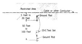
Fig. 7-Two Ground Rod Connection
