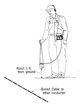
Fig. 8—Locating and Tracing Conductors with the 93B Test Set
