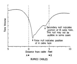
Fig. 12---Two Conductors on Same Route
