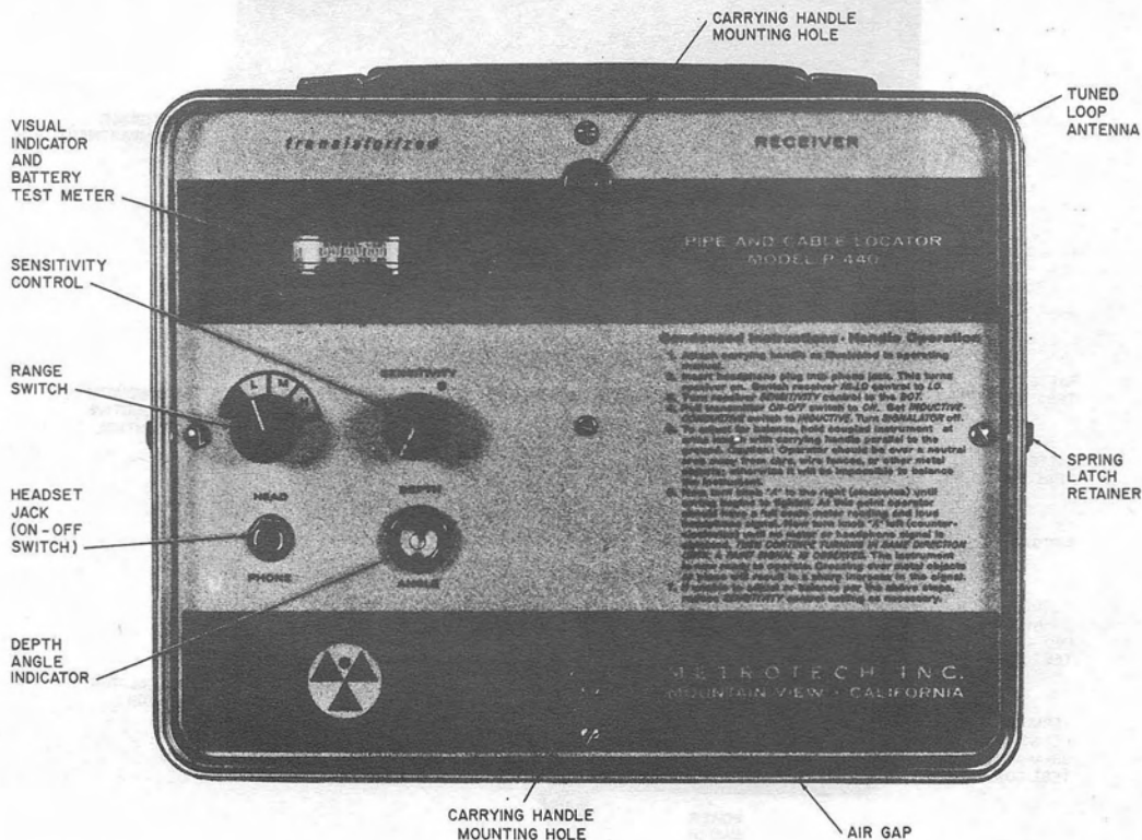
Fig. 14—Receiver Assembly
