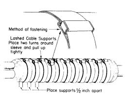
On aerial cable, place cable spacers and support sleeve from strand by applying the end supports in the usual manner. (see section 627–340–101)
