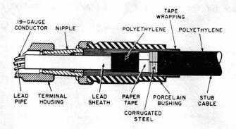
Fig. 2—Bushing Construction of 37B and 37D Terminals
