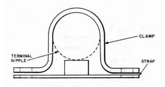
Fig. 5—Hardware for Mounting 37C and 37D Terminals
