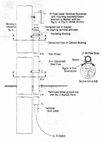
Fig. 6—Steel Pipe Used to Protect Stub Cable
