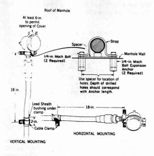
Fig. 8—Mounting Arrangement for Manhole Installation
