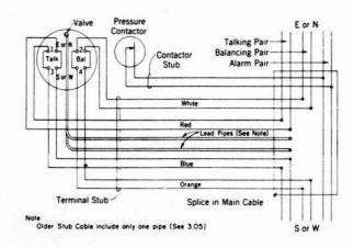
Fig. 12—Balancing Pair Required (Contactor and Terminal Stubs Reach the Main Cable)
