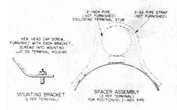
Fig. 4—Hardware for Mounting 37A and 37B Terminals
