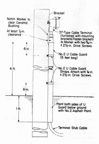
Fig. 7—U Cable Guard Used to Protect Stub Cable
