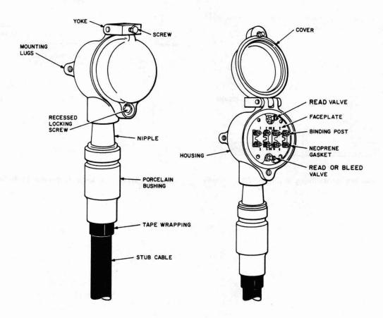
Fig. 3—37B and 37D Cable Terminals
