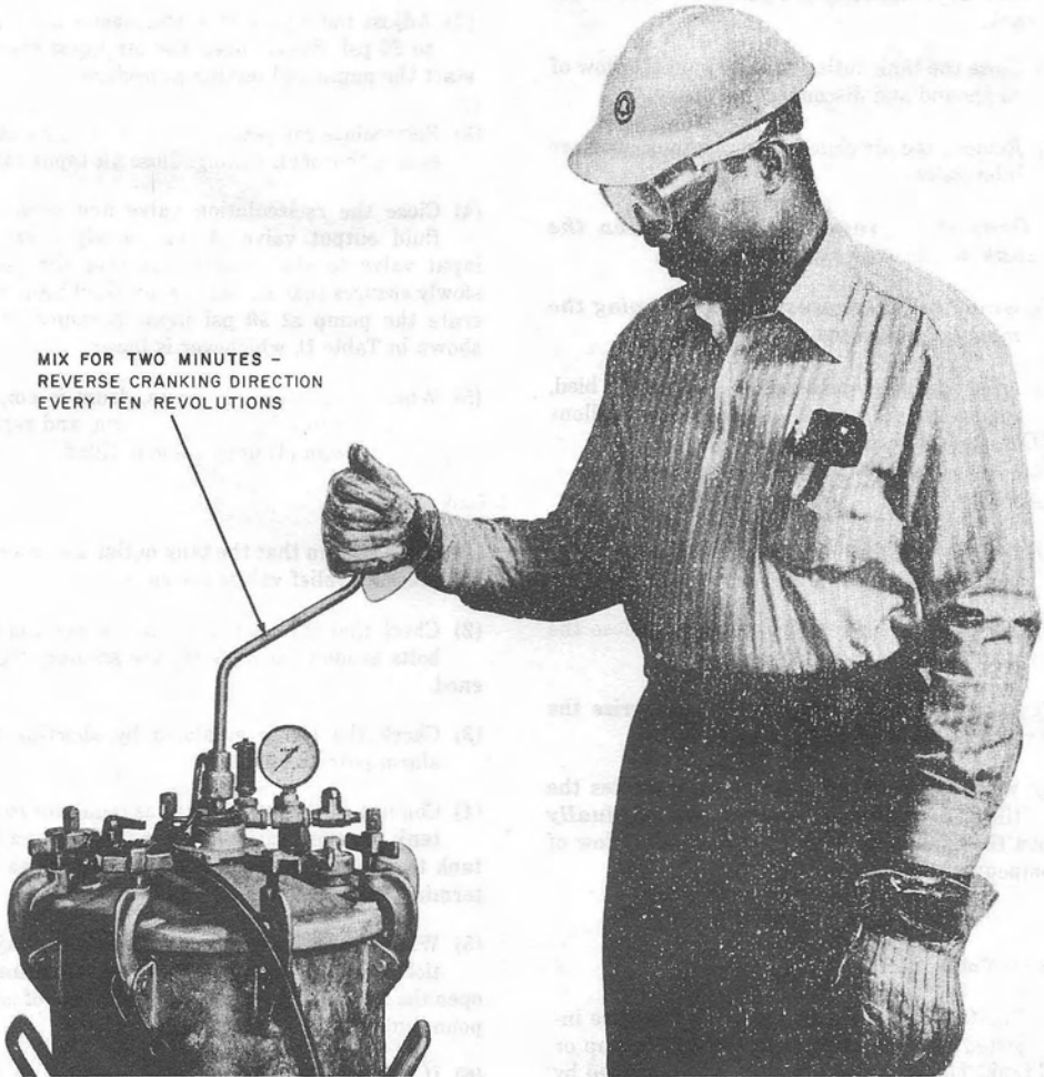
Fig. 15—Mixing C Reclamation Compound—Part I and Part II in C Tank
