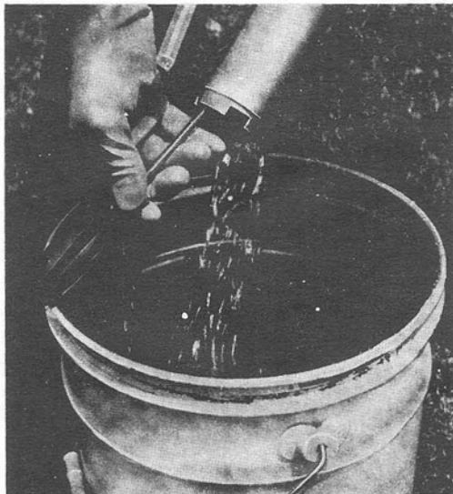
Fig. 18—Draining REN Pump
