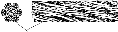
Worn rope, usually indicated by flat spots on the outer wires as shown. This does not apply to type H rope which is designed with flats on the outer wires.
