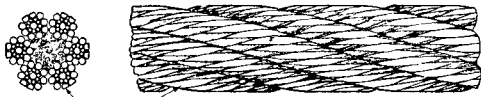
Worn rope, usually indicated by flat spots on the outer wires as shown. This does not apply to type H rope which is designed with flats on the outer wires.
