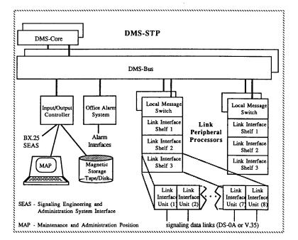
Figure 5. DMS-STP Architecture
