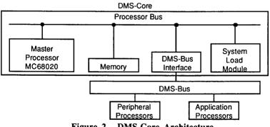
Figure 2. DMS-Core Architecture
