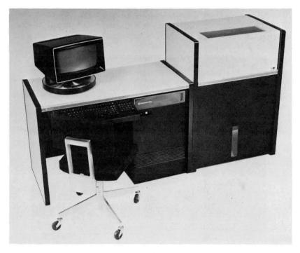
Figure 11-9. A DATASPEED 4540 terminal station arrangement.
