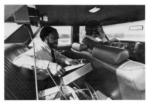
Figure 18-11. Human factors simulation. Laboratory and field simulations play a significant role in the design of user interfaces. Here, human factors engineers use a television camera to study the ease of placing and receiving calls while driving. Tests showed that placing a call with Advanced Mobile Phone Service telephones is as easy as tuning a car radio.
