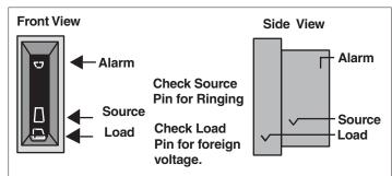
Note: Ringing is a low-frequency AC voltage that may vary during the ringing cycle. Readings of 67 to 155 VAC may be normal. Ringing voltages are superimposed on a DC voltage that can be measured in the DC mode. The DC voltage may 36 to 60 volts. Superimposed ringing may turn positive during part of the ringing cycle.
