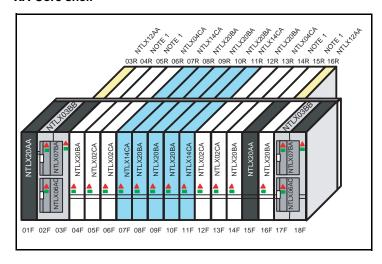
**Note:** Rear slots 4R, 5R, 14R, 15R contain NTLX03AB I/O processors which are populated with NTLX08AB (RTIF) and NTL05AB (CMIC) circuit packs.
