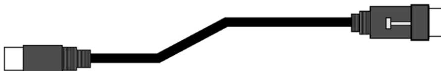
Figure 150 NTAG81CA PC maintenance cable
