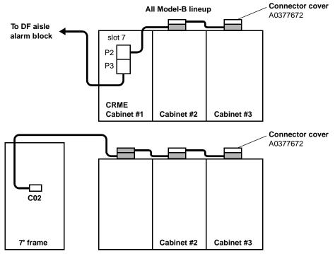
*Note:* In all Model B lineups using a CPDC, the slot number will change from 7 to 5.
