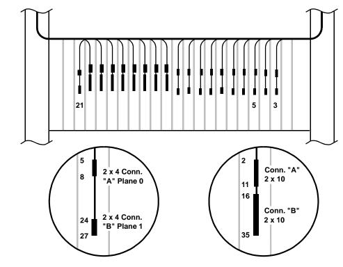
Figure 186 – Connectivity on Backpanel
