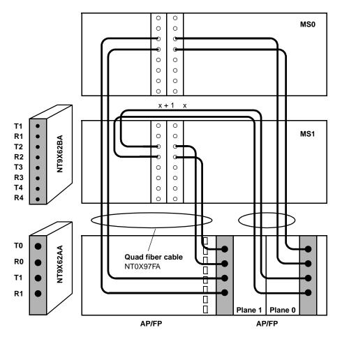
*Note:* Fiber cables are always connected from "Transmit" to "Receive." Refer to cable tags for termination point of each fiber cable.
