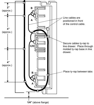
Figure 382 - Rear View of Line Drawer for CLCE
