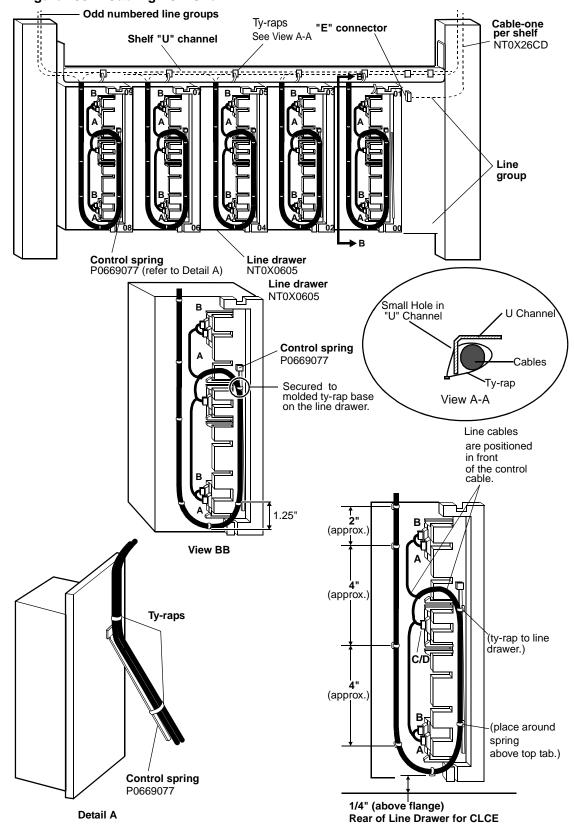
Figure 293 – Cabling LCM Shelf
