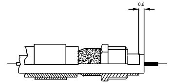
14 Slide the crimp ferrule over the cable braid so that it abutts the hexagonal flange on the rear body and crimp using the Leetec outer crimp tool with the outer crimp die. Refer to Figure 70.
