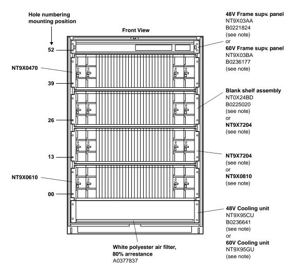
*Note:* NT0X24BD, NT9X7204, and NT9X0810 are provisionable in positions shown and the quantity will vary with provisioning. One of items Cooling Unit or Frame Supervisory Panel is provided per customer requirements.
