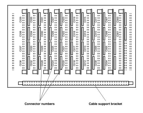
8 The head of the ty-rap is to be located on the opposite side of the bracket as the cable connector. The head of the ty-rap is to be located at the TOP of the connector. Cut the ty-rap flush.
