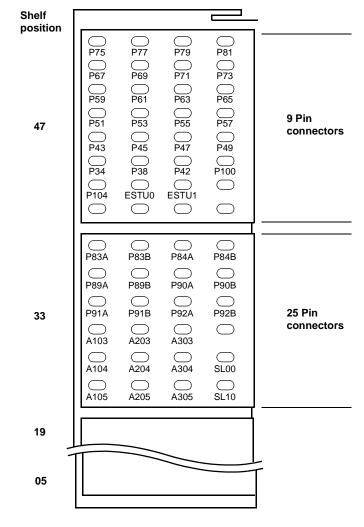
Figure 415 – Bulkhead Layout of CMTA Cabinet
