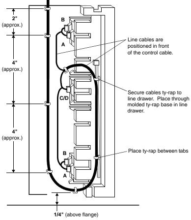
Figure 452 – Rear View of Line Drawer for CRSC (LCM)
