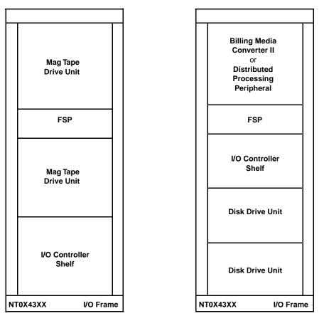
*Note 1:* Mounting positions can vary, see specific procedure for details. *Note 2:* BMC II simplex has only one chassis, which takes up one shelf.
