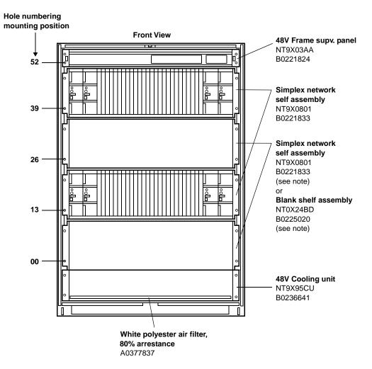
*Note:* NT9X0801 or NT0X24BD may be provisioned at positions 00 and 26. Therefore, quantity will vary from 2 to 4 for NT9X0901, and 0 to 2 for NT0X24BD.
