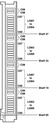
Figure 385 – Model B CLMI Cable Connection Locations
