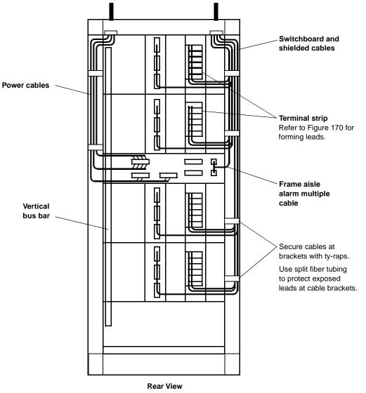
Figure 192 – Cabling and Wiring of the DCE Frame
