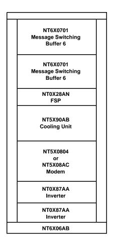
2 The inverter units are not shipped mounted on the frame. They are shipped separately and must be installed onto the frame by the field technician once the frame is in its final place.
