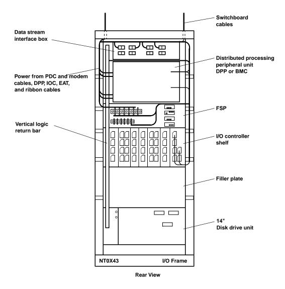
Figure 113 – Typical Cabling Plan - DPPs and BMCs
