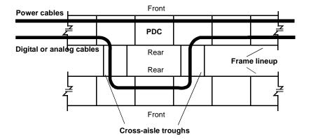
3 When a PDC is installed in the middle of a lineup, plastic protection strips (B0231978, enough for one PDC) must be placed on the trough to protect the cables from sharp edges.
