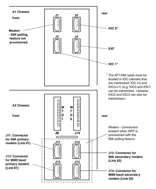
2 The method of connecting the polling modem is dependent upon the baud rate of the modem used and whether the DPP is or is not provisioned with the 56K polling feature. The DPP is equipped with the 56K polling feature if a 56K Interface PCB, NT6M94AA, is located in slots A7 and B7 (refer to Figure 128).
