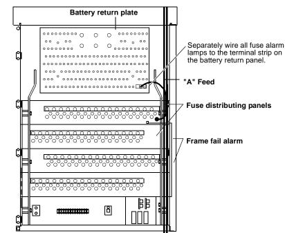
Figure 29 – Fuse Alarm and Frame Fail Alarm Multiple
