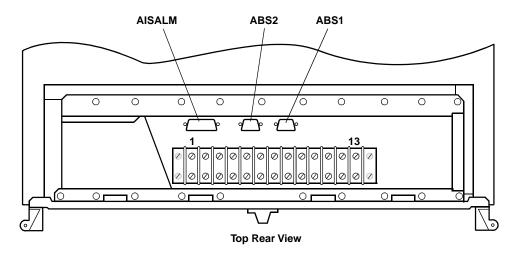
8 Figure 417 reflects the power terminations for the CRSC and CEXT cabinets.
