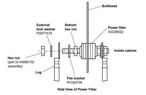
*Note:* Field Technician connections are made on the inside of the EMI cable duct. Torque hex nut to 10 in-lbs. Hold bottom nut while torquing top nut.
