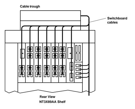
7 When the NT0X46AB frame is provisioned with an NT3X89CA Alarm Cross-connect shelf assembly, the cables are run horizontally under the cable trough and then vertically to their respective connector. Secure the cables with ty-raps at each breakout to metal bar going across top of shelf. Refer to Figure 190. If cables are entering from bottom of frame, use same routing method as when top fed.
