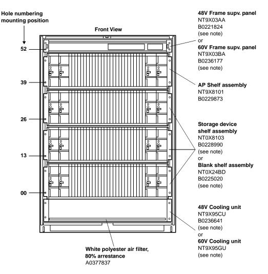
*Note:* NT0X8103 or NT0X24BD may be provisioned at positions 00, 13, and 26. Quantity will vary with provisioning. Only one of items Cooling Unit or Frame Supervisory Panel is provided per customer requirements.
