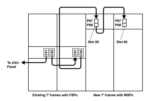
8 On each MSP, there are two loose aisle alarm connectors wrapped with plastic with a small ty-rap. The plastic must be removed on the frame to which the end aisle light will be connected. Connect the cable as shown in Figure 268.
