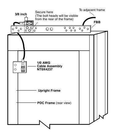
2 Install the NT0X4237 Cable Assembly bolts that secure the #1/0 cable to the adapter plate so that the head of the bolts will be inserted through the adapter plate and then through the cable assembly. The hex nut will be visible from the rear of the frame. Bottom fed configuration requires the NT0X4237 Ground Cable Assembly to be installed at the bottom of the frame.
