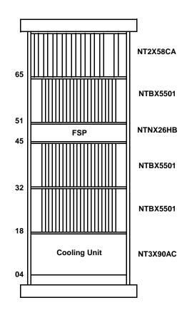
2 The modules will be equipped with circuit packs according to job specifications and requirements. Examples of circuit pack fills are given for the MTM and Remote Line Equipment (RLE) shelves in Figure 307 and Figure 308, respectively.
