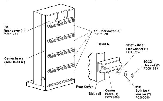
12 Center Brace P0729089 is to be installed as indicated in Figure 87. Split Fiber Tubing P0401296 is to be placed around the Center Brace to protect the local cables where they pass the sharp edges of the center brace. Hold the split fiber tubing in place by securing both ends of the tubing with lacing cord.
