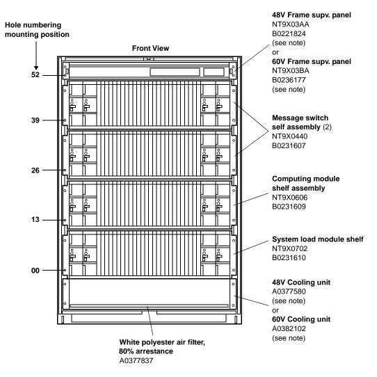
*Note:* Cooling Unit and Frame Supervisory Panel are provisionable and only one each will be required per cabinet.
