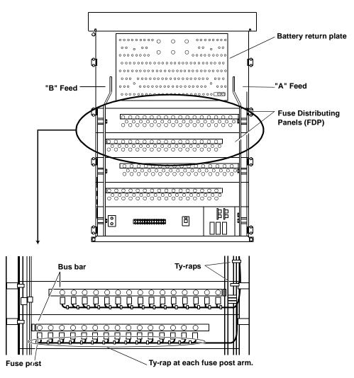
7 Check all torque settings at the inspection torque setting; any screw or bolt found loose must be torqued to the initial torque setting. Any new connection must be torqued to the initial torque setting. Refer to Event 07 (Method 03-9057), "General Cabling and Torque Requirements," for the correct torque measurements.
