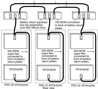
Identify 750 MCM cable ends as"-48V battery return equalizer" using number tags, 145C for U.S. applications or E-8014/E-8015 cable tie markers for Canadian/International applications
