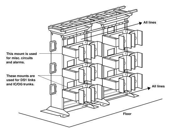
4 Typical layouts of the mounts are shown in Figure 223 and Figure 224. Each job will receive a set of typical and detailed stamping documents -B158.
