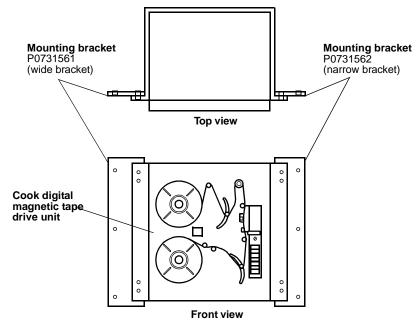
h. Install the rear cover with mounting brackets on the designated frame using mounting screws supplied.
