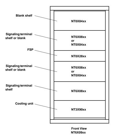
*Note*: The NT6X09AA frame can be provisioned as:
