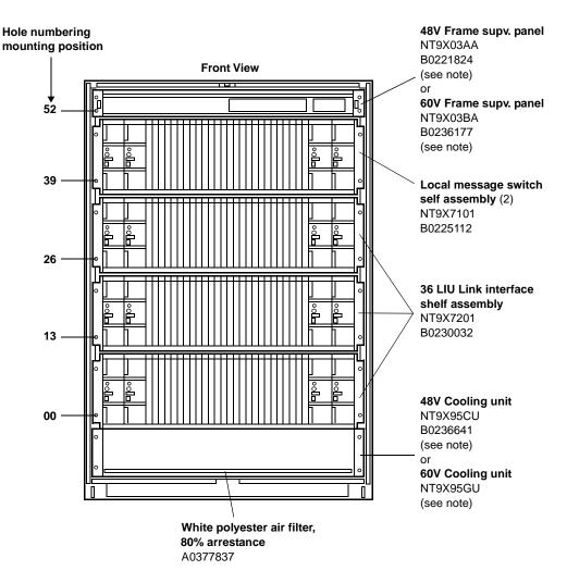
*Note:* Cooling Unit and Frame Supervisory Panel are provisionable and only one each will be required per cabinet. Only one of Cooling Unit or Frame Supervisory Panel is provided per customer requirements.
