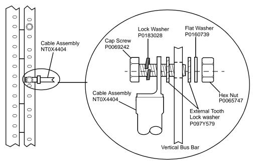
Figure 98 – Ground Terminations at Vertical Logic Bar for Mag Tape Drive
