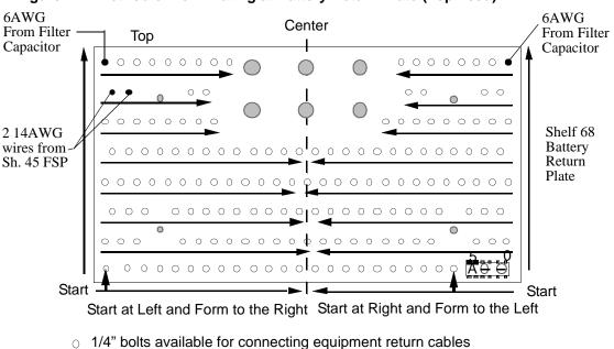
Figure 14 – Method of Terminating at Battery Return Plate (Top Feed)
