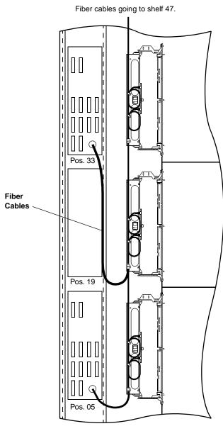
Internal view of bulkhead and backpanel showing FXPM bracket with fiber cables.
