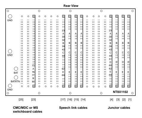
Figure 141 – NT8X1101 Backpanel - Connector Positions
