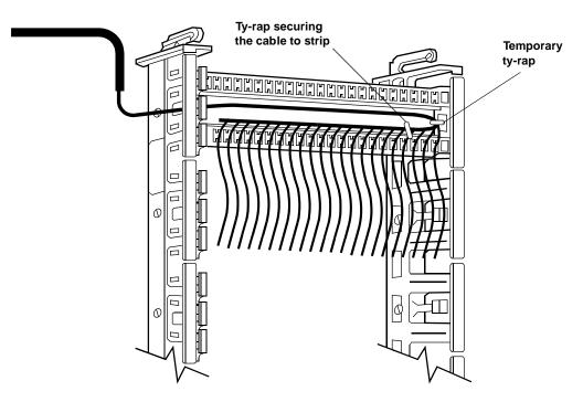
3 Position the strip into place, click it into the BIX mount. At this point the ty-rap holding the cable on the strip is at the right hand side of the mount. Do *not* tighten this ty-rap yet.
