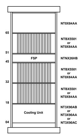
2 An example of a HLE circuit pack fill is given in Figure 238.
