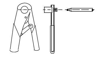
17 Push the assembly fully home, taking up the light spring pressure in the tool and close the tool to crimp the contact in place. Figure 73 shows the assembly as positioned in the Crimping Tool.
