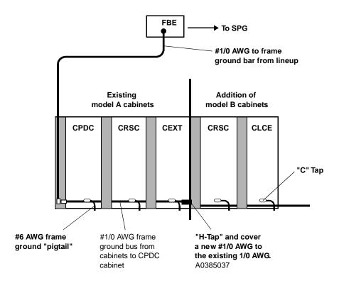
Note: The frame ground pigtail in the C-Tap connection is toward the CPDC.
