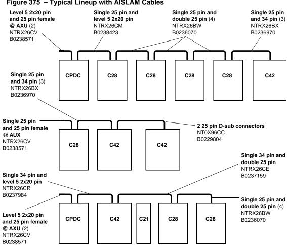
Figure 375 – Typical Lineup with AISLAM Cables
