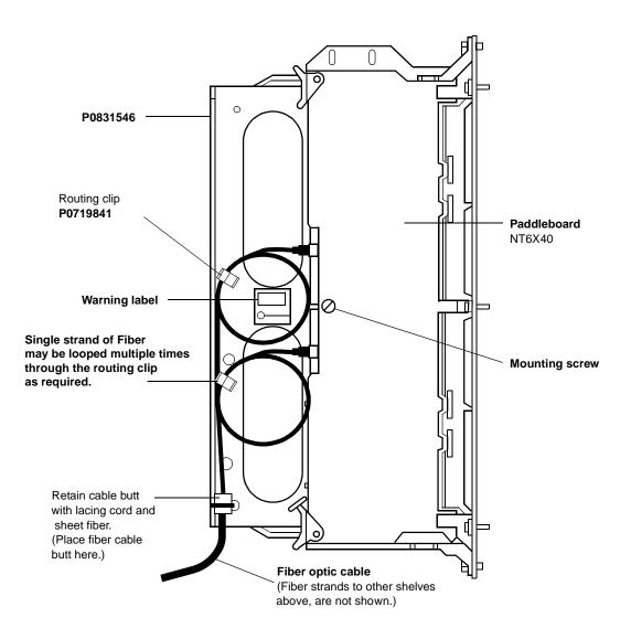
14 Form any excess cable out of the top of the cabinet and secure it to the left side of the bulkhead utilizing sheet fiber and lacing cord. Use a "Kansas City Stitch" to secure the cable to the bulkhead.
