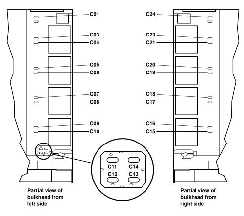
*Note:* Cxx refers the feed thru capacitor number. Refer to the labels on the bulkhead for the product specific A or B designations.
