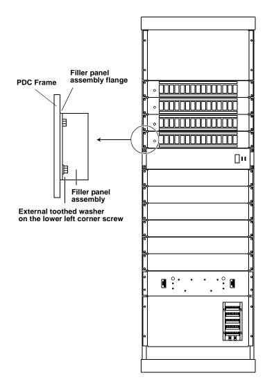
7 Secure the fuse panel in place with the four 5/16" self tapping screws which were previously removed from the filler panel assembly. Use 1/4" drive torque wrench (T0179) to torque the screws to 50 in-lbs. Refer to Event 07 (Method 03-9057), "General Cabling and Torque Requirements."
