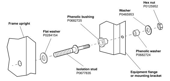
3 Figure 164 shows the mounting hardware for the modified equipment where the normal mounting screw can be used with the isolation hardware.
