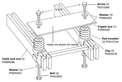
*Note:* Mount this assembly above each PDC Frame requiring modification. This assembly may be mounted above or below the ladder rack.
