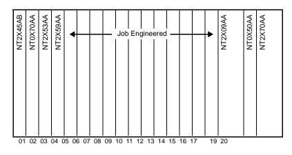
Figure 308 – Remote Line Equipment (RLE) Shelf Circuit Pack Fill
