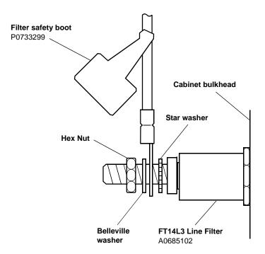
*Note:* The Filter Safety Boot is part of NT9X9545 (B0234548) consisting of 22 Safety Boots. Hex nut and washers are part of A0685102 FT14L3 line filter assembly. The hex nut and washers can only be obtained with the line filter. These parts are not available separately. P0730273 boots may be provisioned with NT9X70BB only for use with 6 or 8 AWG power feeders. When using P0730273, discard P0733299 provided as part of NT9X9545.
