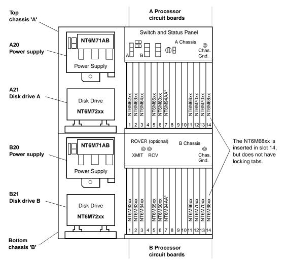
Figure 397 – DPP Cabinet Subassemblies Front View (Covers Removed)
