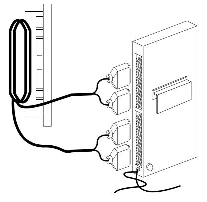
Figure 83 – Tester B, Connection of Main Unit Directly to Subgroup Cables
