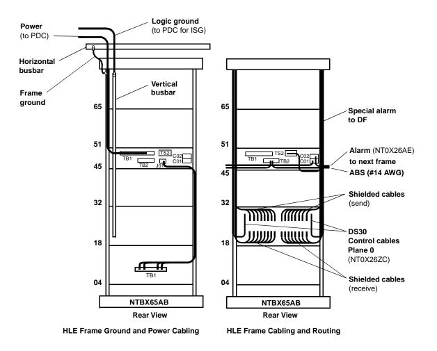
2 Connect the cable braid assembly from the top of the frame left upright (rear view) to the third hole from the left end (rear view) of the bar.
