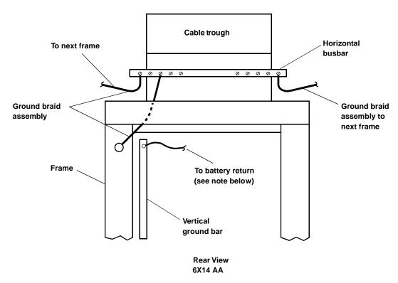
*Note:* If FSP NT6X25AA, then connect to TB2-9 (left). If FSP NT6X25BA, then connect to TB1-4 (bottom). Both connections are factory installed.
