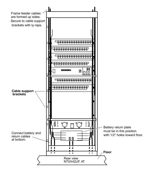
2 For bottom mounted, bottom feed, battery return plates, secure the 750/500 MCM battery return cables to the battery return plate as shown in Figure 9. If only one cable is installed per mounting hole, install the cable to the inside of the frame.
