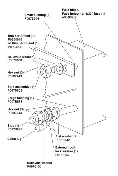
9 Refer to Figure 12 for the hardware stackup for fuse positions found in the non-UL approved fuse panels. Non-UL approved fuse blocks are NT0X42AB/AC.
