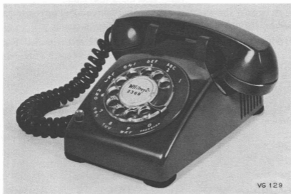
FIG. 1-23. Low-current tone ringer telephone set.
