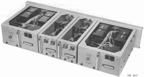
FIG. 5-20. Power supplies and paralleling units.
