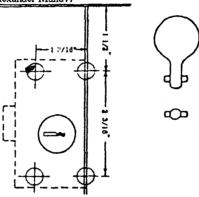
After this is accomplished, the lock can be pushed backwards, disengaging the lock from the cover plate. The four bolts of the cover plate can then be retracted by turning the boltworks with a simple key in the shape of the hole of the coin plate. Of course there are other methods and drilling patterns.
