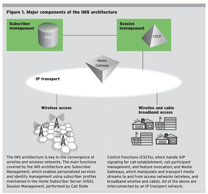
single, unified services model that is much more powerful than that of the telephony network. Moreover, SIP supports the establishment of bidirectional media streams between users and between an application server and user. Unlike web-style invocation of an application server, which must be client initiated, SIP enables push services, where an application server makes the call to a client.
