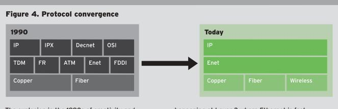
The explosion in the 1990s of creativity and invention in networks created a large number of competitive (or at least co-existent) protocols and media/control. During the late 1990s, organizations converged on IP as the common Layer 3 protocol, and within enterprise campuses Ethernet became the dominant solution. The same convergence is
