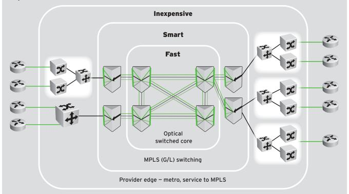
This diagram depicts an architecture for the future that distinctly separates the metro transport and the long-haul transport domains. In this architecture, service management is at the provider edge, while the metro transport network is optimized for speed without being burdened by the complexity and intelligence necessary to provide large-scale
