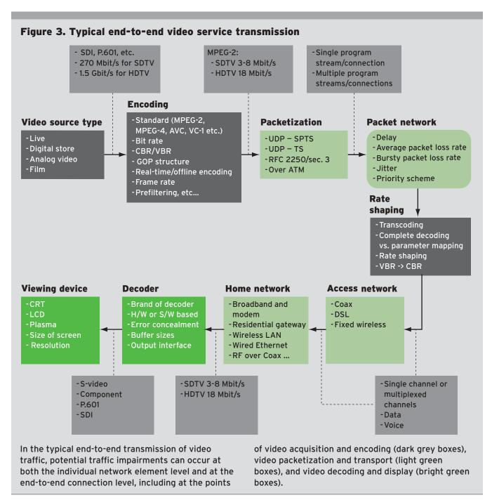
set from an end-to-end perspective – from the video head-end to the set-top box.
