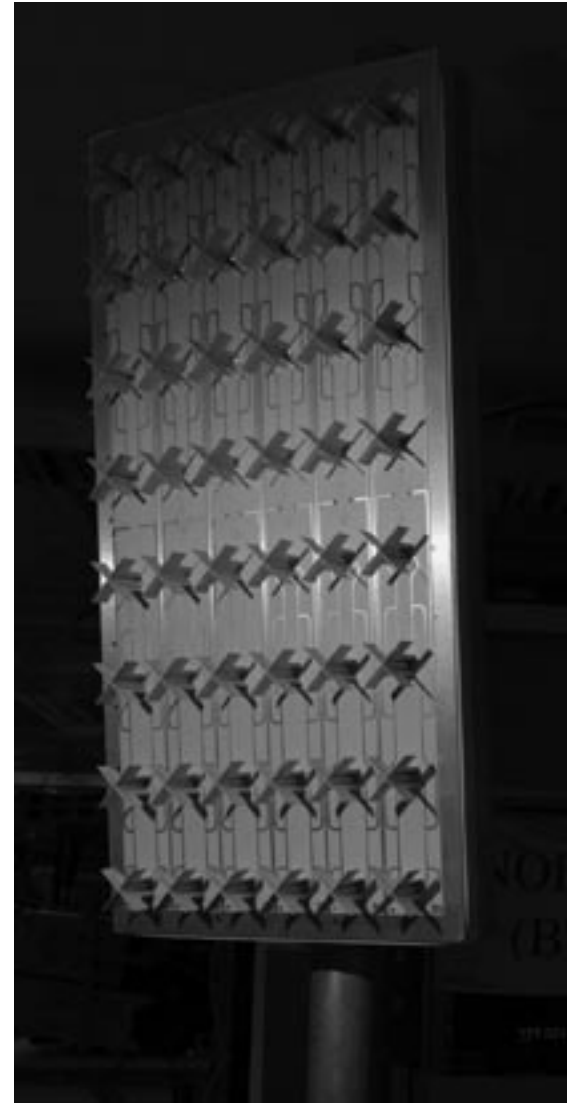
Pictured above is a prototype of a Nortel-developed MIMO base station antenna. This particular antenna configuration shows polarization diversity – that is, two arrays of antenna elements that are co-located and oriented orthogonally, at 90 degrees to each other. In other words, all the antenna elements that slope downward comprise one MIMO antenna array; all elements that slope upward form another – effectively combining two antennas in one, giving double the efficiency with the same-sized antenna and increasing coverage, which is particularly beneficial for challenging radio propagation environments, such as dense urban areas. For more, see page 24.
