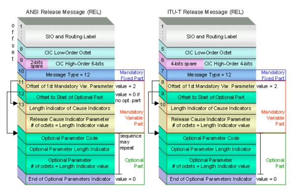
Figure 13. ANSI and ITU-T Release (REL) Message Format
