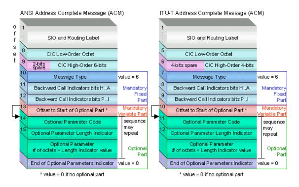
Figure 11. ANSI and ITU-T Address Complete Message (ACM) Format
