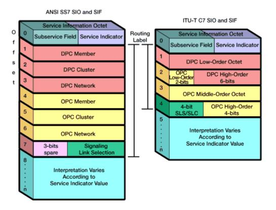
Figure 7. ANSI vs. ITU-T SIO and SIF
