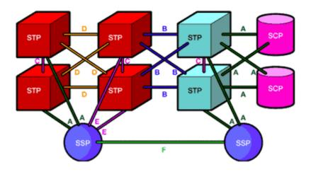
Figure 2. SS7 Signaling Link Types
