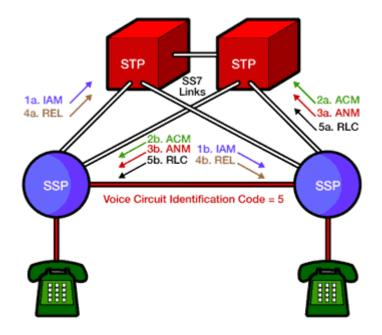
Figure 8. Basic ISUP Signaling
