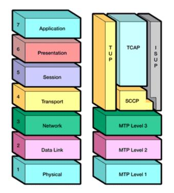
Figure 3. The OSI Reference Model and the SS7 Protocol Stack
