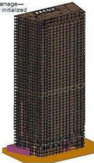
Figure 12-33. Debris impact damage application to the global LS-DYNA model.
