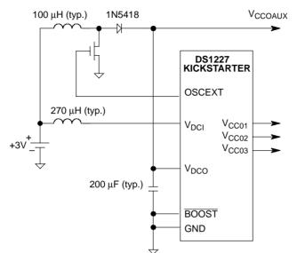
The DC-DC converter's output current is provided both by the inductor and directly from the battery. If the load draws less than the maximum current, the  $V_{DCI}$  n-channel MOSFET is turned on only often enough to keep the output voltage at the desired level.
