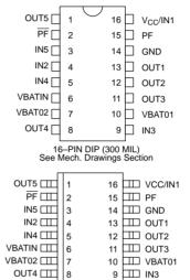
16-PIN SOIC (300 MIL) See Mech. Drawings Section
