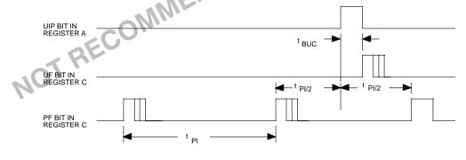
$t_{PI} = \text{Periodic interrupt time interval per Table 1.} \\ t_{BUC} = \text{Delay time before update cycle} = 244 \ \mu\text{s.}$
