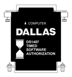
tion to the number, serialize media and absolutely trace field units. The 4096 bits of read/write memory are organized in 16 pages of 256 bits each. An additional scratch page is provided to assure data integrity before any writes to nonvolatile memory take place.
