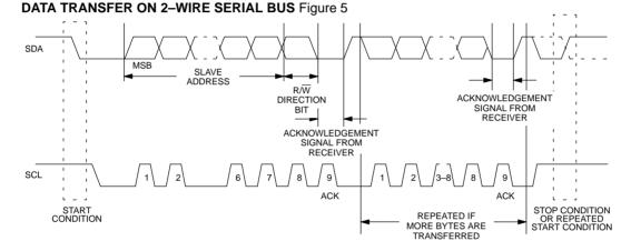
Figure 6 details how data transfer is accomplished on the two–wire bus. Depending upon the state of the R/W bit, two types of data transfer are possible:
