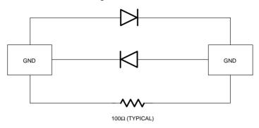
**NOTE:** GND and AGND must be tied to the same voltage level.
