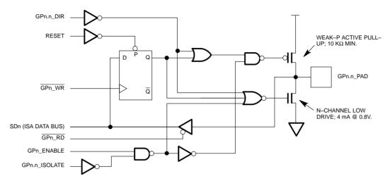
As stated above, each pin can be individually programmed to perform as an input only, input/output, or electrically isolated from the system (high–Z).
