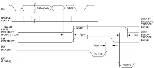
RECEIVER FIFO FIRST BYTE TIMING Figure11-22
