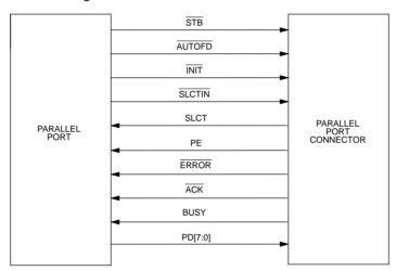
The following general protocol is used when communicating with a printer or other parallel port device.
