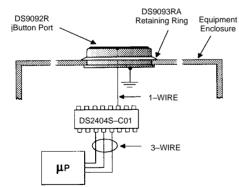
Equipment fitted with 1-Wire button contact.
