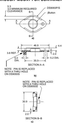
The DS9093S and DS9093P allows the user to permanently attach an <u>i</u>Button to an object with one or two screws, rivets, etc. The plastic plate is designed with an inset that accommodates the flange of the F5 package and allows for flush mounting. A protective wall
