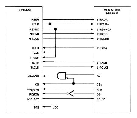
\*HDLC on the FDL can be implemented either by the second serial input (TDM CHANNEL B) or via the port by the host processor (CPU32 internal to the QUICC32).
