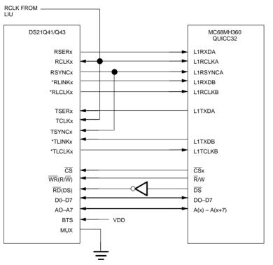
\*HDLC on the FDL can be implemented either by TDM CHANNEL B or via the port by the host processor (CPU32 internal to the QUICC32).
