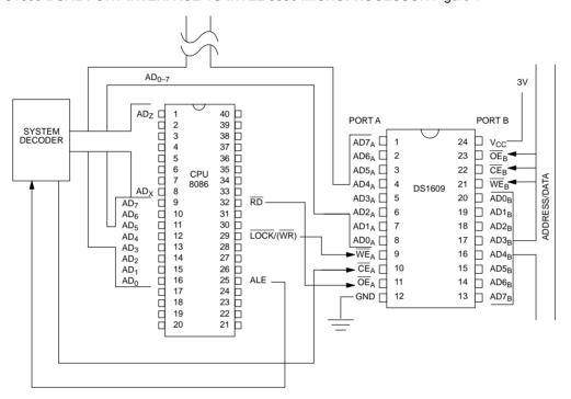
The DS1609 is ideally suited for small microprocessor based systems which frequently utilize dedicated 8 bit multiplexed address/data busses the following examples deal with interfacing with the Intel 8086/8088 series and the Motorola HC11 series microprocessors.
