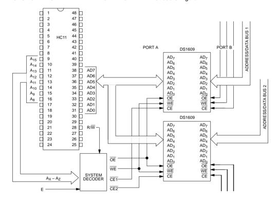
The DS1609 can be used as a go between with non-multiplexed microprocessors such as the Intel 386 or Motorola 68030. Processor cycles to and from a
