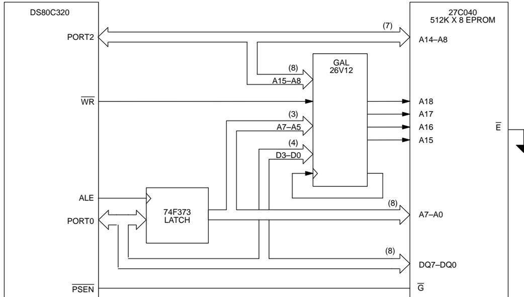
The following software example shows an assembly language routine to jump to a new location in any bank using latched data as shown in Figure 6. Before calling the bank switch subroutine, software pushes the new address and bank number onto the stack. It then calls a
