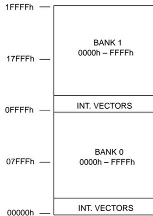
This approach is most effective when page switching is kept to a minimum, i.e. executing straight runs of code. Code efficiency will be improved if the interrupt routines (not just the vectors) are small enough to be duplicated on each page as well. Data tables or strings accessed with MOVC instructions should be located on the same page as the instruction.
