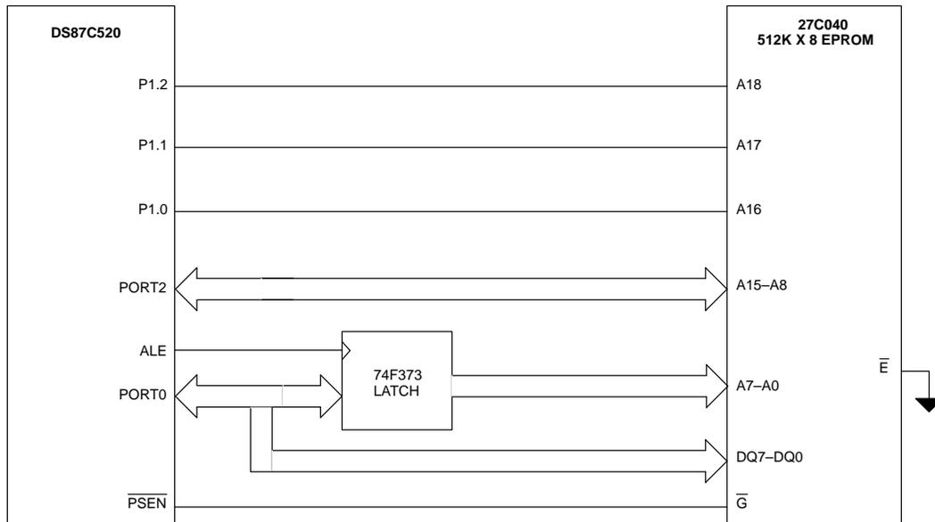
Expanding the amount of data memory used by the microcontroller is the easiest form of memory expansion. Because there is no possibility of interfering with program execution, timing is not as critical. General purpose I/O lines can be connected directly to the address lines or chip enables of the memory device(s). The
