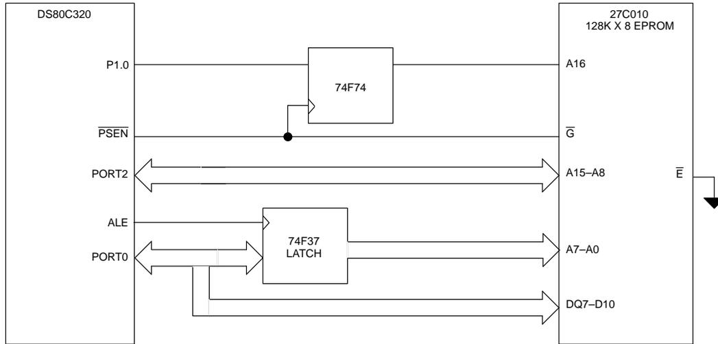
The simplicity of the hardware comes at the cost of some software complexity, however. This example uses two banks, both of which contain the interrupt vector tables in the lower portion of memory. This is necessary because when the device is reset, P1.0 will be high, forcing the reset vector address to 10000h. Also, an interrupt may occur while executing code from either
