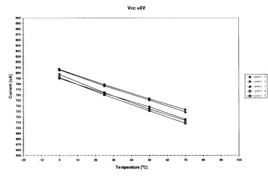
$V_{CC}$  = +3.0 and +5.0 volts. The DS1802 configuration for this test has no activity on 3-Wire serial ports, push-
