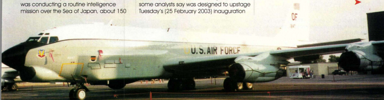
RC-135U, distinctive with the forward nose cameras. The side 'Chipmunk Cheeks' are electronic signal collectors (referred to as 'Rivet Joint' used to collect signals intelligence). The RC-135S, has fuselage mounted windows for cameras to take long-range photographs of incoming missile re-entry vehicles (RVs). The RC-135U on display during Ellsworth Air Force Base's open house and air show, Dakota Thunder 2000 (August). Photograph: Lieutenant Colonel George A. Larson, USAF (Ret.)
