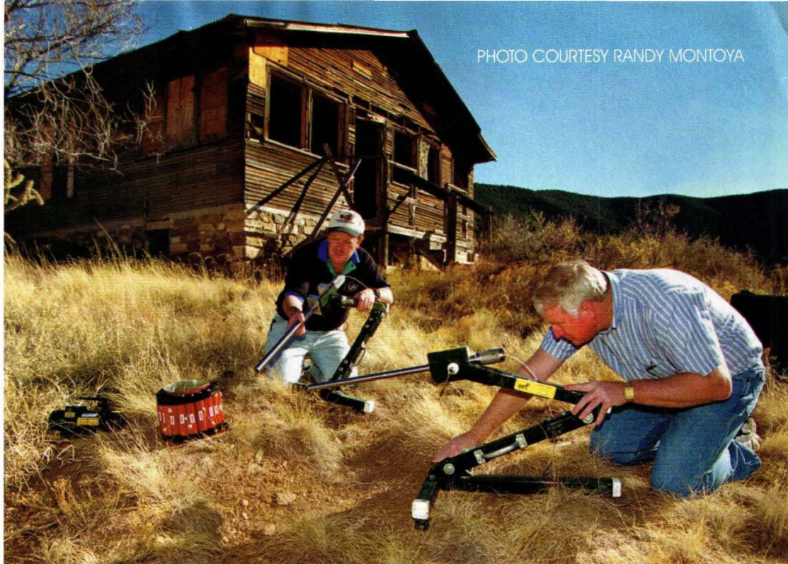
Sandia National Laboratories bomb-disablement experts Chris Cherry (right) and Rod Owenby demonstrate use of two PAN Disrupters on a mock bomb
