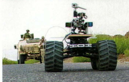
The multi-functional advanced remote control, or MARC Bot, tackles improvised explosive devices
