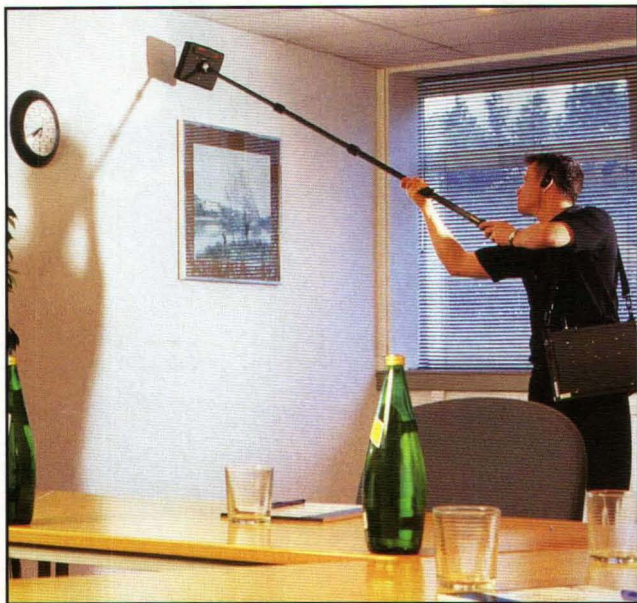
AUDIOTEL's 'Superbroom' will detect transmitting and non-transmitting bugs
