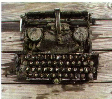
The typewriter that was attached to M2946 as a printing device. A fragment of the connecting cable is visible at lower left
