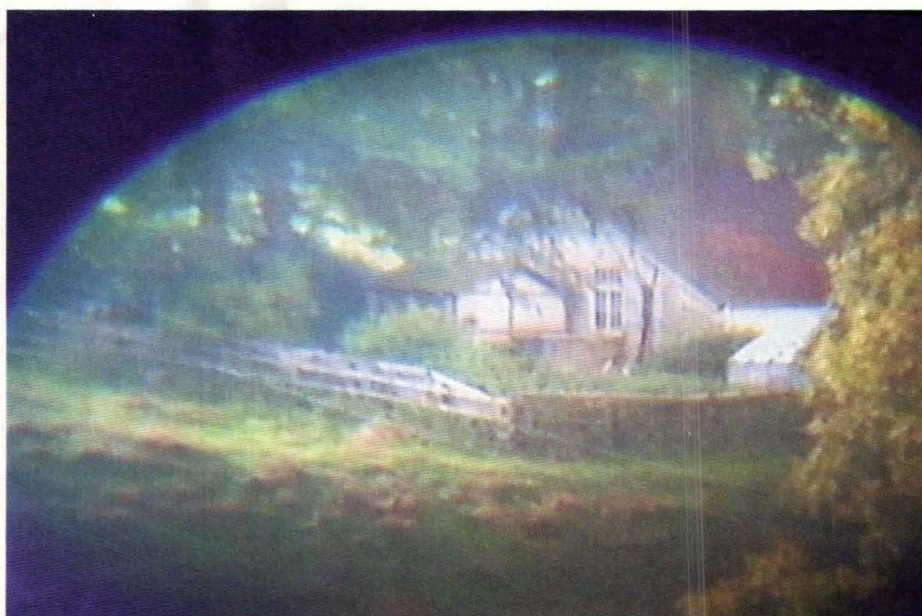
An untouched screen shot from our monitor after the camera was attached to the binoculars. The dark arch is caused by the caps
