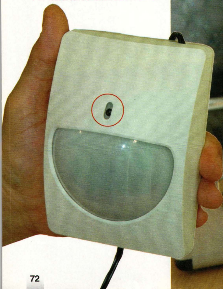
3G camera with audio installed inside PIR - ideal for constant surveillance
