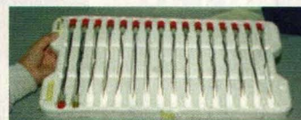
Above: Exploding-bridgewire detonators in case
