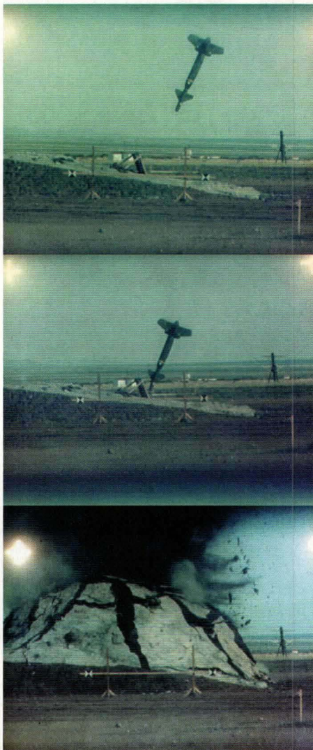
Test firing. A GBU-24 Paveway III missile sinks inside this structure before exploding
