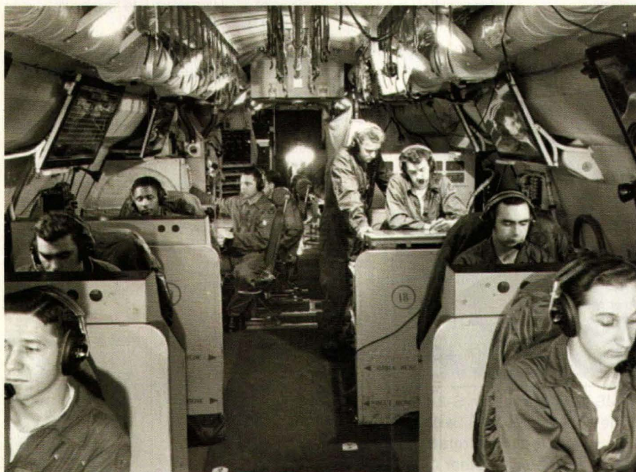
Radar operators and intelligence personnel on a USAF Lockheed EC-121D Warning Star. 552nd Airborne Early Warning and Control Wing
