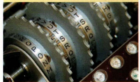
Rotor wheels from a German Enigma
