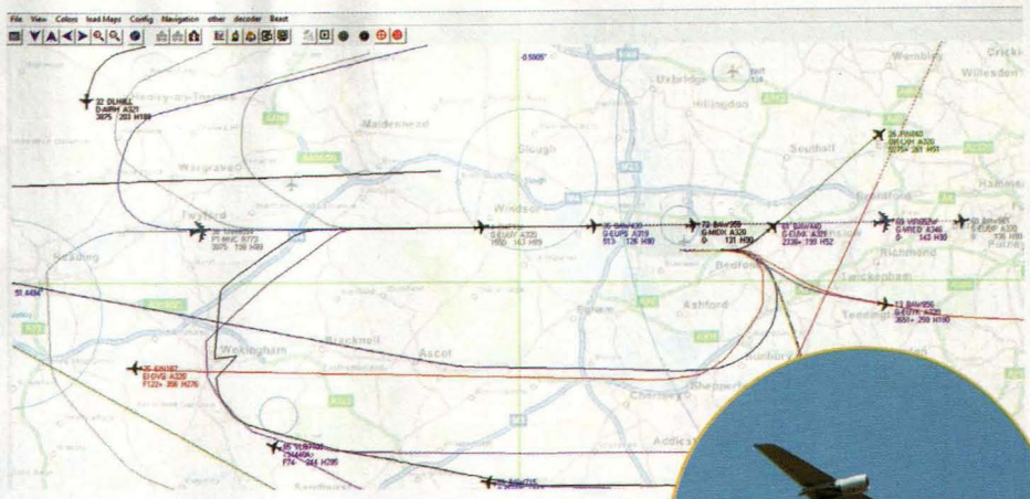
Emerging technologies allow for the reception of Mode S transponder transmissions - thus the tracking of commercial aircraft
