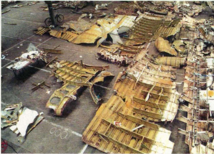
Debris from Pan Am Flight 103 was taken to a warehouse by air crash investigators at Longtown, Cumbria (left). What remained was transported to Air Accident Investigation Branch at Farnborough, Hampshire and reassembled (right)
